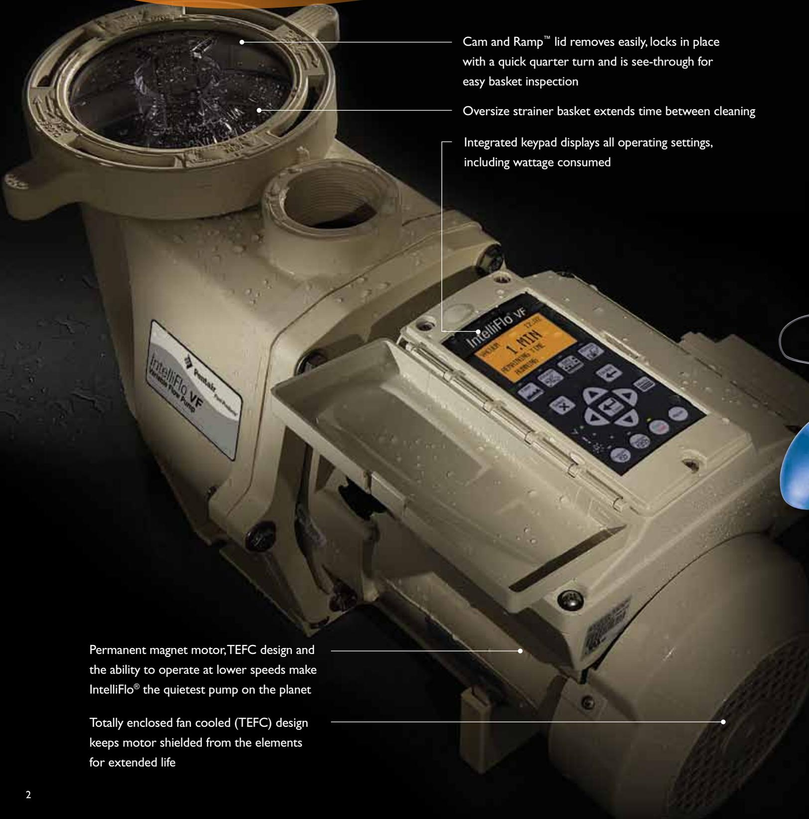
Cam and Ramp™ lid removes easily, locks in place with a quick quarter turn and is see-through for easy basket inspection
