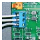
Figure 1. Remote Pool-Off Spa Connection (3-Wire Connection)
