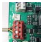
Figure 3. AquaLink RS 485 Communication (4-Wire Connection)
