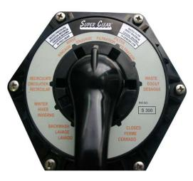
**Filter** – Water travels from pool thru sand filter bed and returns to pool. Used to filter pool water and while vacuuming pool. **Backwash** – To clean filter sand. Turn pump off, set multiport valve to backwash, restart pump for several minutes or until site glass shows clear water. Then rinse filter.(see Rinse below).
