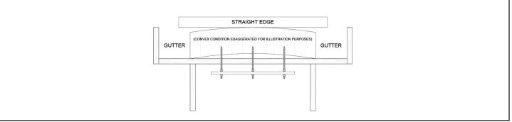
To correct a concave playfield, loosen the nut below the metal bar. Slowly tighten the nut above the metal bar down against the bar in order to push the center of the playfield up.
