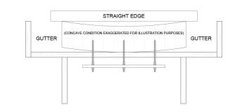
Once the desired adjustment has been made, continue to the next Climatic Adjuster and repeat the process.
