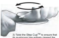
its mushroom has entirely cleared the wall thickness. If it has, the suction cup should rotate freely.
