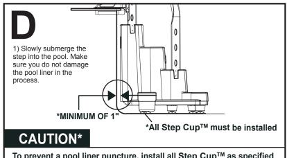
To prevent a pool liner puncture, install all Step Cup™ as specified and keep a minimum of 1"inch gap between the pool liner and the rear underside of the step.
