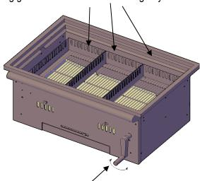
Rotate the height adjustment knob to adjust the charcoal bed for multi-level heat control
