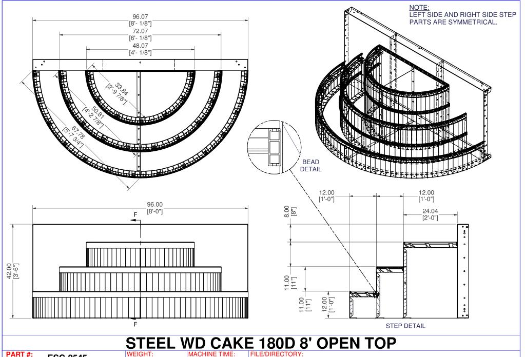
PART #: **ESC-2545** I:\PRODUCT CATALOG\2015 SS\ESC-2545.idw 319.90 lbmass N/A MATERIAL: DATE: TOLERANCES EXCEPT NOTES: 8/3/2015 AS NOTED DRAWN BY: SHEET: 2 OF 4 RP ±1/8 ±0.25 ±0.0625 ±0.03125 ±1/2°
