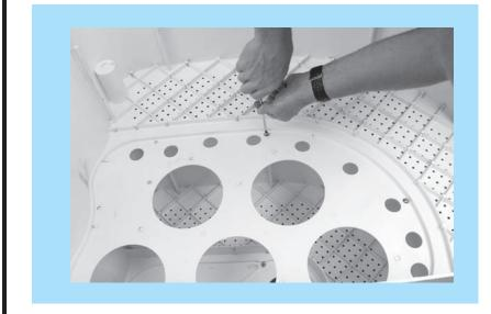
• Be sure to secure step 3 to the assembly using all 6 stainless steel screws and washers.
