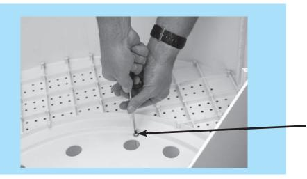
• Make sure you fasten step 3 to step 2 at all 6 points using a stainless steel washer with each screw.
