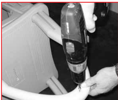
#10: Overlap the flat sections at top of the handrails and connect using 1-#10 x 1-1/4" self tapping screw. Repeat for other handrail.
