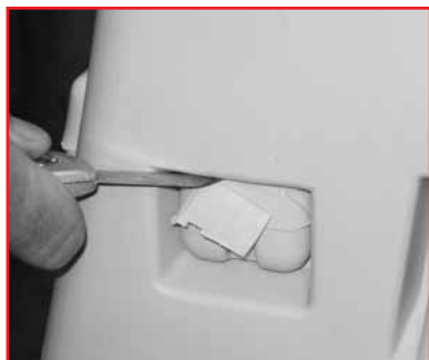
#9: Using a sharp knife carefully cut off the plastic tabs.
