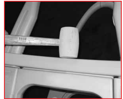
#9: Finish tapping deck all the way down until engaged on to bridge.
