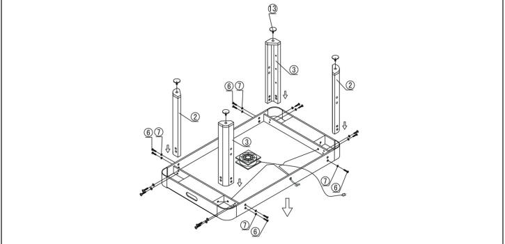
3. Attach each LEG PANEL #4 to LEGS as shown with SCREW #10. Note: Graphics should face outward.
