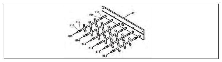
4. Insert PLAYER RODS through holes on other SIDE PANEL and attach to each END PANEL with CORNER #17 and 1/2" SCREW #4 as you did in step 1.
