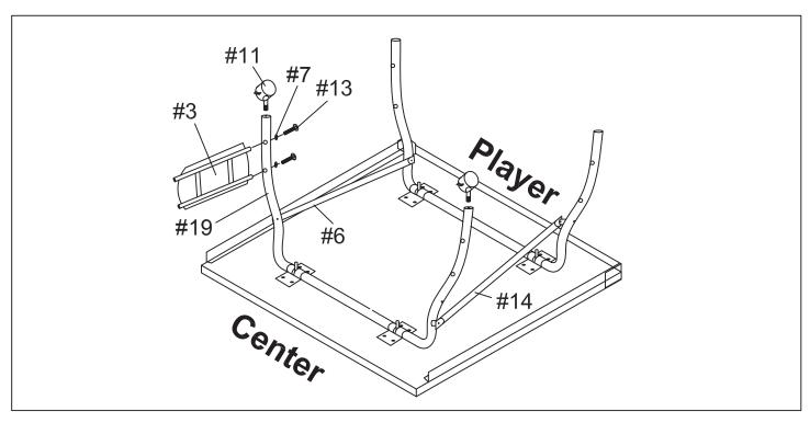
5. Carefully turn the two table surfaces over and attach the PLASTIC PLATE WITH STEEL FRAME, #3, to the opposite table leg, as shown, with BOLTS, #13, and WASHERS, #7.
