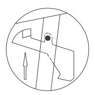
Move up the safety lock, so it catches the bottom of the table, when folding up for storage. Move down, to disengage table, before opening the tables for play.
