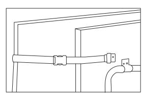
Clip the strap buckles together when folding the two table tops for storage. *Note: Remove Net Posts and Net, and store in bag, before folding table for storage.*
