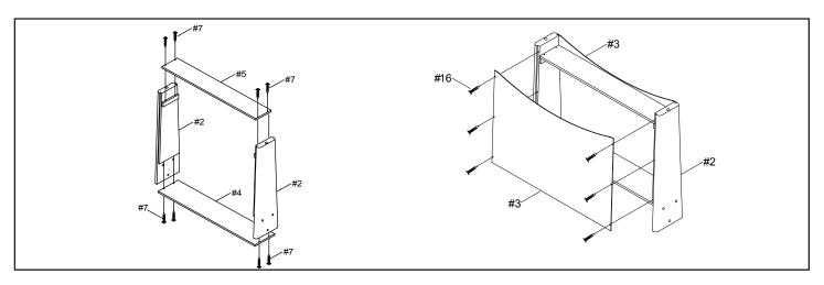
Note: The Leg assembly may require two individuals, one to hold pieces, while the other inserts screws. TIP: If you hand insert all screws, on a single piece, into pre-drilled holes before tightening, it will help hold the pieces in alignment as you tighten the screws.
