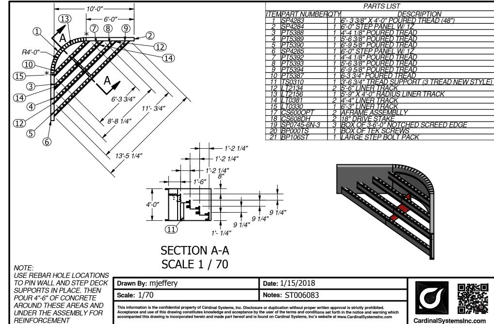
5'-6" LINER TRACK <u>5'-9" X 4'-0" RĂDĬÛS LINER TRACK</u> 4'-4" LINER TRACK 6'-3" LINER TRACK AFRAME ASSEMBLL 18" DRIVE STAKE 3 BOX OF 3-6-0" NOTCHED SCREED EDGE 1 BOX OF TEK SCREWS LARGE STEP BOLT PACK
