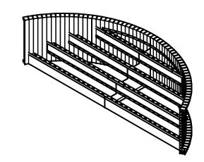
NOTE: USE REBAR HOLE LOCATIONS TO PIN WALL AND STEP DECK SUPPORTS IN PLACE. THEN POUR 4"-6" OF CONCRETE AROUND THESE AREAS AND UNDER THE ASSEMBLY FOR REINFORCEMENT
