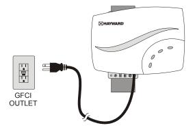
After being powered on for the first time, the Salt & Swim 3C will run a diagnostic routine which can take up to 30 seconds. During this time, various LEDs will turn on and off. When finished, the Salt & Swim 3C will display a blinking INADEQUATE WATER FLOW LED and a solid STANDING BY LED. Keep the Salt & Swim 3C powered for the remainder of this procedure and go to Step 3.
