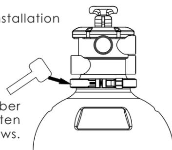
tap with a rubber mallet and tighten the screws.
