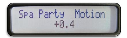
Note: When motion is set to OFF, there is no delay and all lights will illuminate at the same time. When motion is set to a positive value (+0.2 to +1.2), the order of illumination will start from the lowest LT number and advance to the highest. If a negative motion value is selected (-1.2 to -0.2), the illumination sequence will be the opposite (highest LT to lowest).
