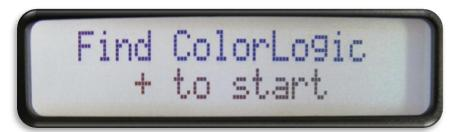
Note: Once the ColorLogic configuration process begins, there is no way to exit and the process must be completed.
