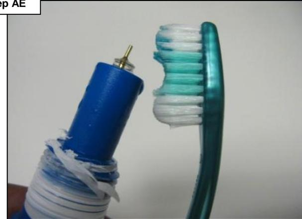
Follow the steps on page 4. Once probe is clean run the filter pump for 2 hours. Check readings. If the value continues to remain low, despite high free chlorine in the pool, then replace the probe (GLX-PROBE-ORP).
