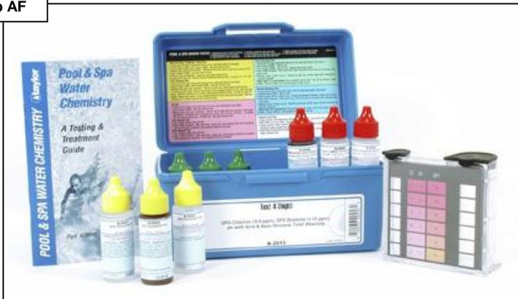
It is important to test the chlorine level of the water in the flow cell as well as the water in the pool. If chlorine levels are high in both the pool and flow cell, then lower the ORP set point or lower the chlorinator percentage. If the chlorine level are high in the flow cell only go to step AG. If the chlorine levels are normal/low go to step AH.
