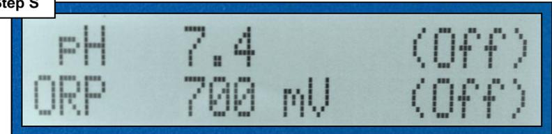
If attached to a ProLogic follow instructions on page 5. If attached to an Aqua Rite Pro follow instructions on page 6. After recalibrating the probe, if the variance between the independent test and the system's reading is more than 10% different, then replace the pH probe.
