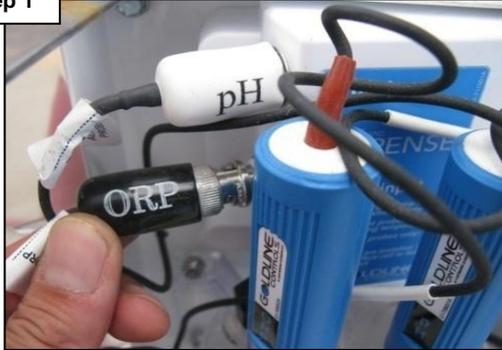
Disconnect the probe connectors from the flow cell.
