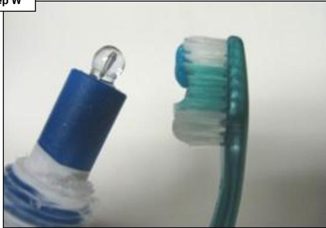
Follow the steps on page 4. Once probe is clean run the filter pump for 2 hours. Check readings. Recalibrate (page 5-6). After recalibrating the probe, if the variance between the independent test and the system's reading is more than 10% different, then replace the pH probe.
