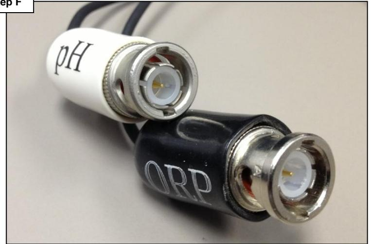
If the connectors are clean replace the probe that corresponds with the error (GLX-PROBE-PH) or (GLX-PROBE-ORP). In some rare cases the problem can be caused by a bad module (GLX-SD-ELEC-MOD).
