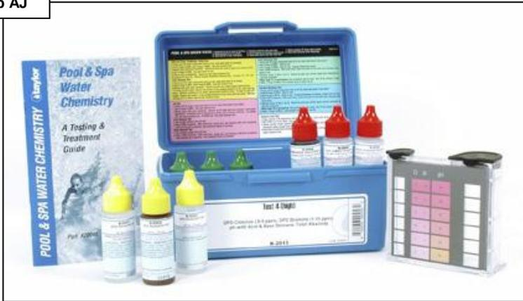
Measure the complete water chemistry, including phosphates and stabilizer, using an external test kit to ensure the water is balanced. Balance the water if needed. If chlorine levels are low put the system in 'Chlorine Feed – Timed %' and 'Super Chlorinate' of a minimum of 24 hours. If chlorine levels still remain low go to AK. If chlorine levels are high go to step AM.
