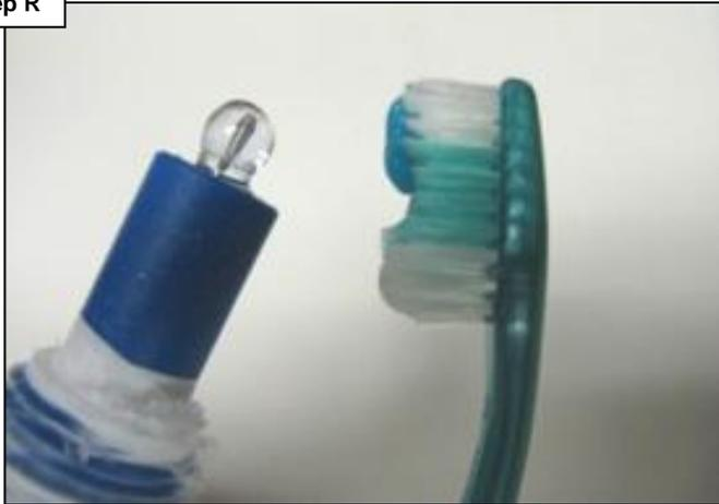
Follow the steps on page 4. Once probe is clean run the filter pump for 2 hours. Check readings. If the readings are not accurate within 10% go to step S.
