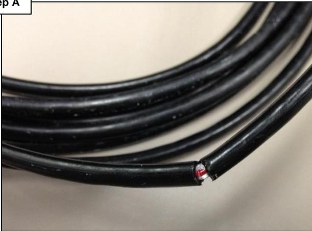
If the cable is damaged then it will need to be replaced. If the cable does not have any damage, go to step B.
