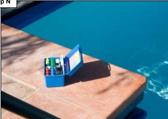
It is important to test the pH value of the water in the flow cell as well as the water in the pool. If pH is high in both the pool and flow cell, add muriatic acid to lower and go to step P. If the pH is high in the flow chamber only, go to step O. If the pH is not high at all go to step R.
