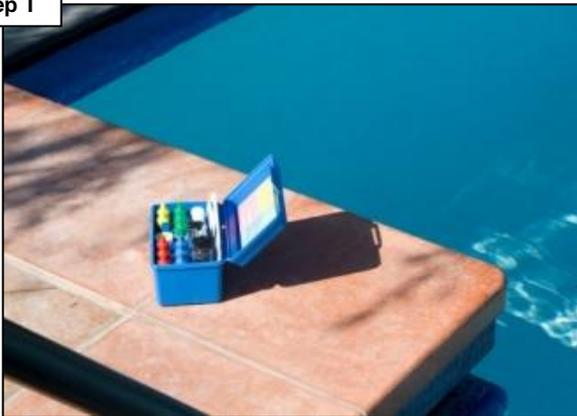
It is important to test the pH value of the water in the flow cell as well as the water in the pool. If pH is high in both the pool and flow cell, add muriatic acid to lower and go to step U. If the pH is high in the flow chamber only, go to step V. If the pH is not high at all go to step W.
