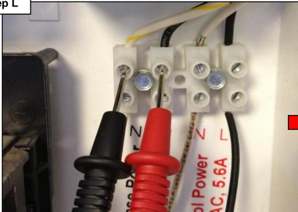
If the voltage is present then the pH reduction circuit has been compromised and the main board will need to be replaced (GLX-PCB-PRO or GLX-PCB-AR-PRO). If voltage is 0 and CO<sub>2</sub> is being used, go to step M.
