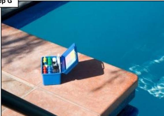
It is important to test the pH value of the water in the flow cell as well as the water in the pool. If pH is low in both the pool and flow cell, add soda ash to raise and go to step L. If the pH is low in the flow chamber only, go to step H. If the pH is not low at all go to step J.
