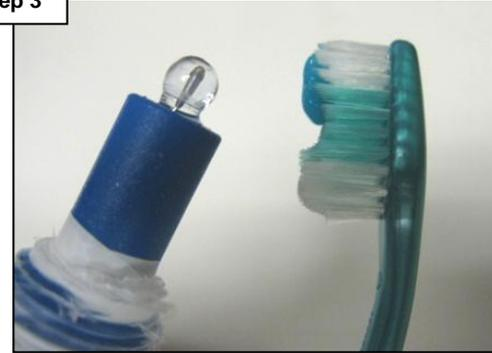
Clean the probe tip and white reference area with a soft tooth brush and regular toothpaste or liquid dish washing detergent.
