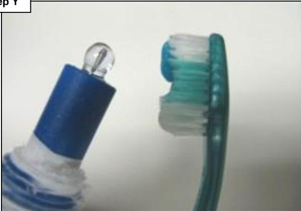
Follow the steps on page 4. Once probe is clean run the filter pump for 2 hours. Check readings and go to step Z.
