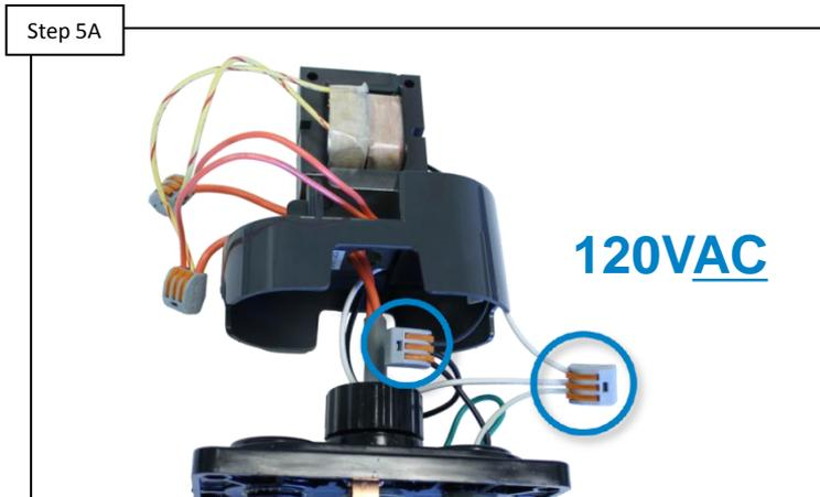
Verify that the transformer has 120VAC on the primary side. IF NO voltage is present, correct source power issue (tripped GFCI, Light relay not engaged...etc.). IF voltage is correct, go to step 5B.
