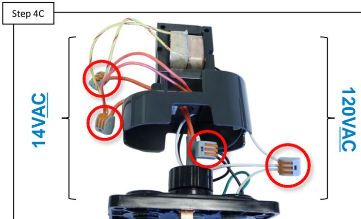
Verify that all connections in the junction box are secure and measuring correctly. IF connections are not correct, secure them and retest. IF connections are secure, proceed to step 4D.
