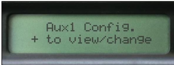
Once complete, navigate to each relay you wish to control the lights through by pressing the (>), press (+) to enter each relay.
