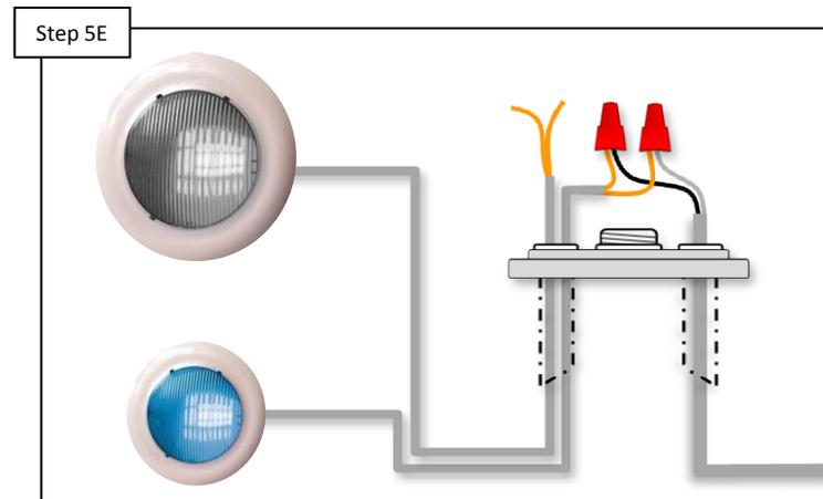
**Isolate each light one at a time, IF all lights work individually, then voltage drop or overloading are likely playing a factor. IF only certain lights are working, replace any faulty lights.**
