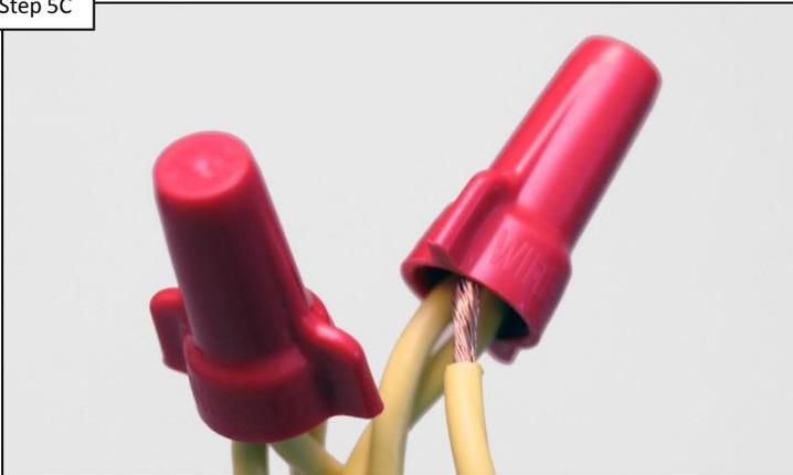
Inspect any junction points for poor connections. Check voltage, verifying 12-14VAC is present. IF connections are correct, go to step 5D. IF NOT, correct and/or replace damaged or faulty wiring.
