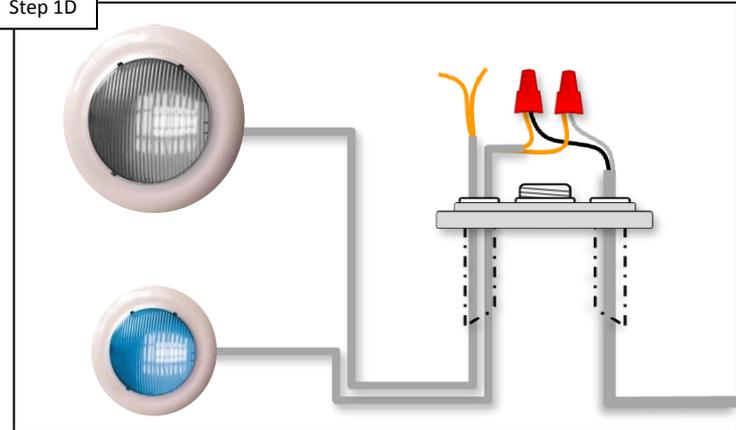
Isolate each light one at a time, IF all lights work individually, then voltage drop or overloading are likely playing a factor. IF only certain lights are working, replace any faulty lights.
