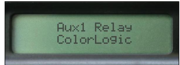
Press the (>) to locate the relay type and change it to "ColorLogic" by pressing the (+), then press (>) to assign lights.
