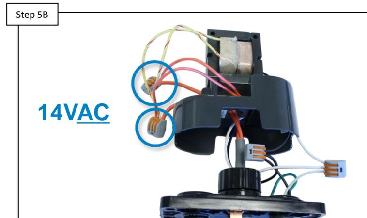
Verify that the transformer has 14VAC on the secondary side. IF NO voltage is present, verify connection and replace transformer if necessary. IF voltage is correct, go to step 5C.
