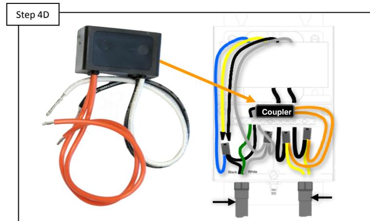
Each transformer used for network lighting should have its own coupler (this boosts the communication). IF any couplers are missing, install them ([LKBUN1000](#)). IF all transformers have network couplers, go to 4E.
