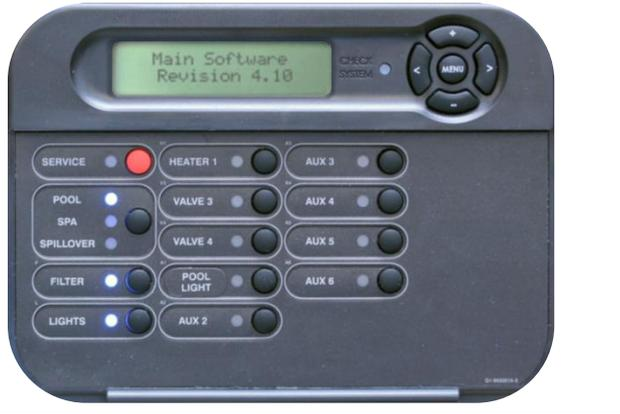
Verify the main software rev. of the ProLogic is 4.10 or higher. This can be found in the back of the Diagnostic Menu. IF correct go to, 7B. IF incorrect, replace the main board with a newer version ([GLX-PCB-PRO](#)).
