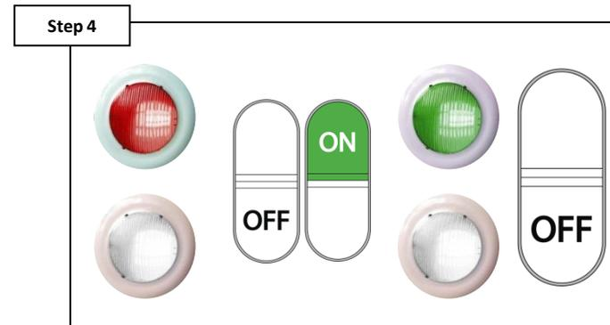
To change modes, quickly turn light OFF then right back ON. Once mode is correct, keep OFF for 2 minutes to lock it in.
