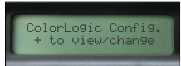
Press the (>) until "ColorLogic Config." appears on the screen, then press the plus (+) to enter.
