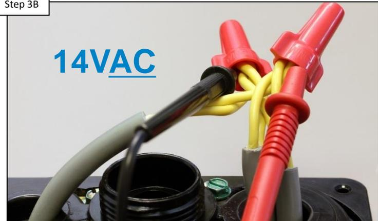
The LED(s) will flash if not enough power is being supplied. Verify power is 12-14VAC at the junction point. IF no/low voltage, go to step 3C. IF correct, check connections and call tech support (908) 355.7995.
