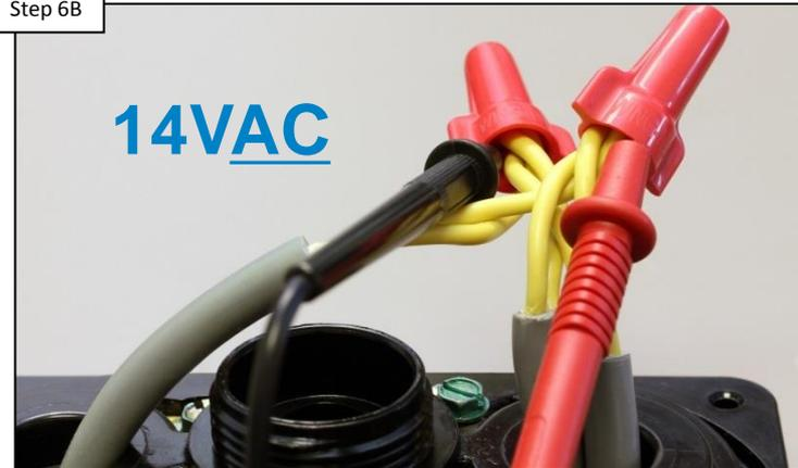
The LED(s) will flash if not enough power is being supplied. Verify power is 12-14VAC at the junction point. IF no/low voltage, go to step 6C. IF correct, check connections and call tech support (908) 355.7995.
