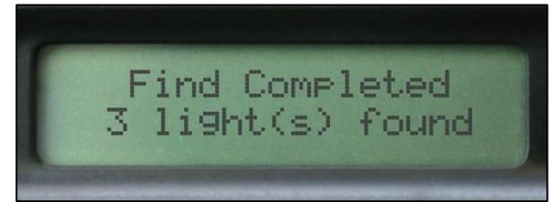
Once complete, press the (>) and assign each light a number using (+) & (-) NOTE: recommended for advanced programming.
