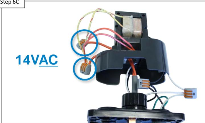
Verify that the transformer has 14VAC on the secondary side. IF NO voltage is present, go to step 6D. IF voltage is correct, there is a break in the line, a bad connection, OR a voltage drop issue.
