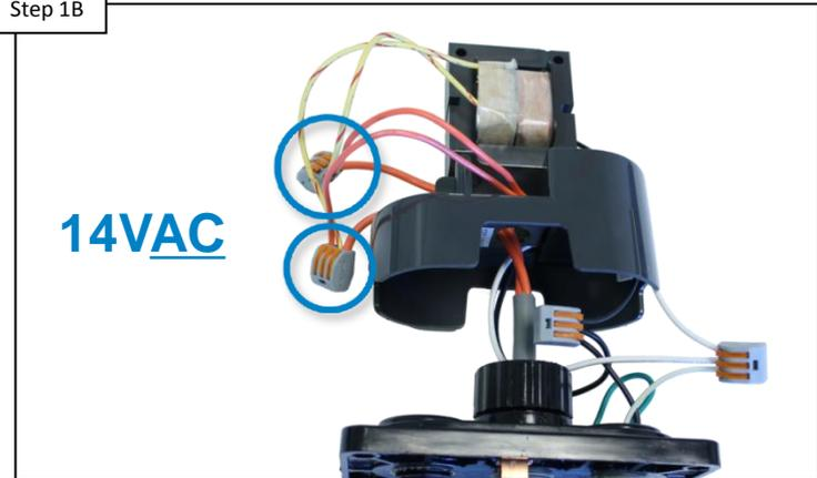
Verify that the transformer has 14VAC on the secondary side. IF NO voltage is present, verify connection and replace transformer if necessary. IF voltage is correct, go to step 1C.
