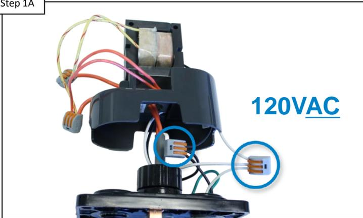
Verify that the transformer has 120VAC on the primary side. IF NO voltage is present, correct source power issue (tripped GFCI, Light relay not engaged...etc.). IF voltage is correct, go to step 1B.
