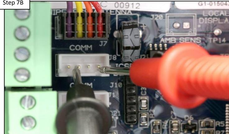
Test the comm port (bus) where the module plugs in for 9-14VDC between pins 2 & 4 (left to right). IF the voltage is correct, skip directly to step 7D. IF incorrect, proceed to step 7C.
