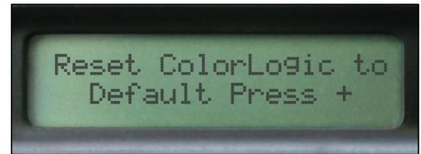
Press the (<) until "Reset ColorLogic to Default." appears on the screen, then press the plus (+) to enter.
