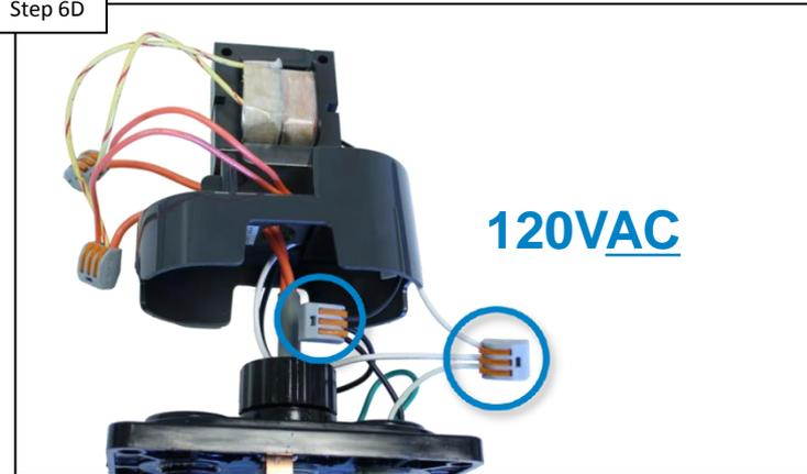
Verify that the transformer has 120VAC on the primary side. IF NO voltage is present, correct source power issue. IF voltage is correct, check connections then replace transformer if necessary.
