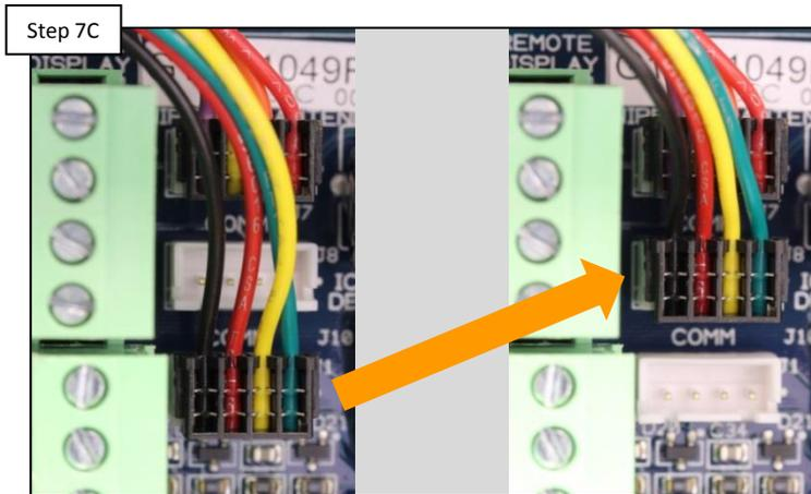
Move the network module's communication connector to an open port. IF no open ports are available OR moving it does not correct the problem, replace the main circuit board (GLX-PCB-PRO).
