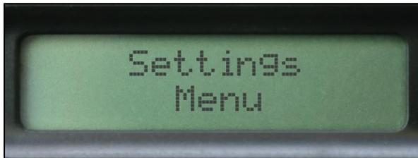
Once all the desired relays are set to "ColorLogic", press the "Menu" button until the "Settings Menu" appears.
