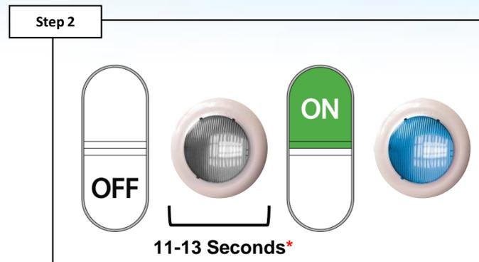
Turn OFF the light off for 11-13 seconds\*, then immediately back ON.
