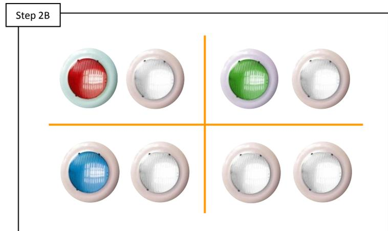
Verify the light mode of each light (pg. 10). IF any of the lights are not in the same mode, correct this (pg. 11). IF lights are all in the same mode, go to step 2C.
