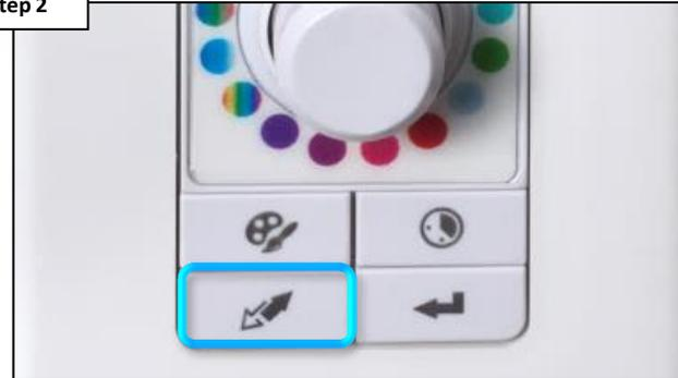
Wait 2 minutes then press and hold the resync button for no less than 3 seconds.
